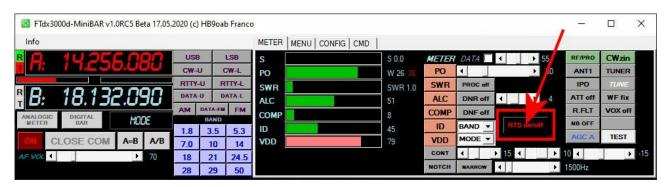
With this APP home made I can quickly activate and deactivate the status of the RTS both on the RADIO and in the SOFT, keeping the signal HIGH or LOW (true or false), RTS & CTS necessary if it is activated on the radio to start or stop data transfer.
