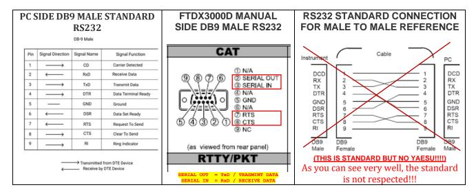
To better verify, in addition to measuring the outputs of the levels, I used my own application (FTdx3000d MiniBar) that I configured specifically with the signals:
